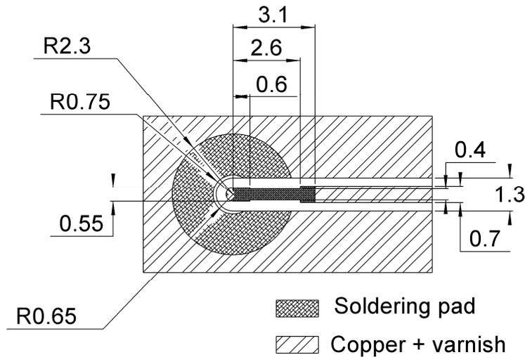
Substrate: RO4350 thickness 0.254mm, with copper layer 35µm on both sides:
